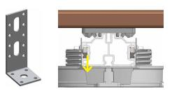
The characteristic strength of the bolt in the rail is: Fax,Rd = 3383 N
