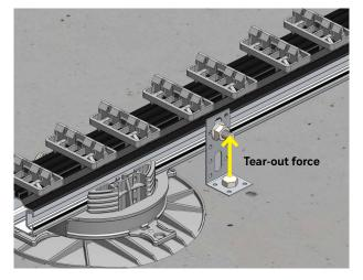
Use an angle bracket or steel strip with M8 bolts to anchor the deck to the ground. Fastening is staggered, and the number of anchors per  $m^2$  can be determined by taking into account the uplift force due to wind and the deck's own weight.
